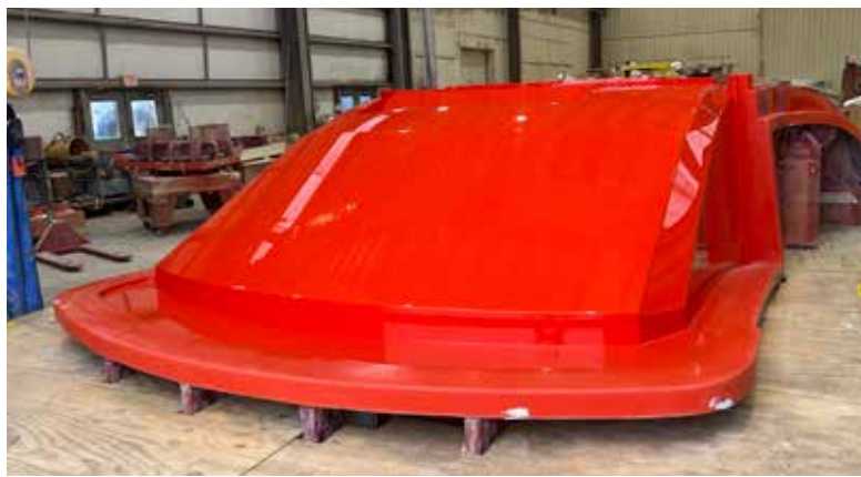
Left: The pilothouse lower liner mold is buffed and polished before the fiberglass team begins part production.
