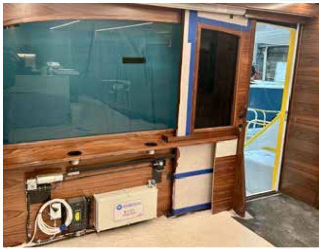
A Marine Power Door system on the bulkhead of a Viking 82 before final finish work conceals the components.
